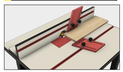
For the cleanest cuts and crisp edges, use a feather board to hold the stock to the router table's surface, and another to press the work into the fence. Feed segments face down for 12-sided objects at a slow and steady rate. A push stick will provide maximum control and will keep your hands at a safe distance from the router bit.
